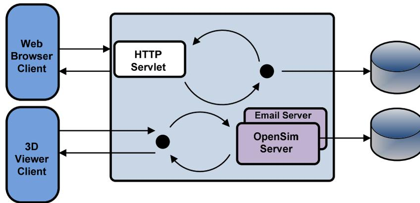
**Figure 3 Top-level view of the architecture of our system which is based on a 3D virtual platform**
